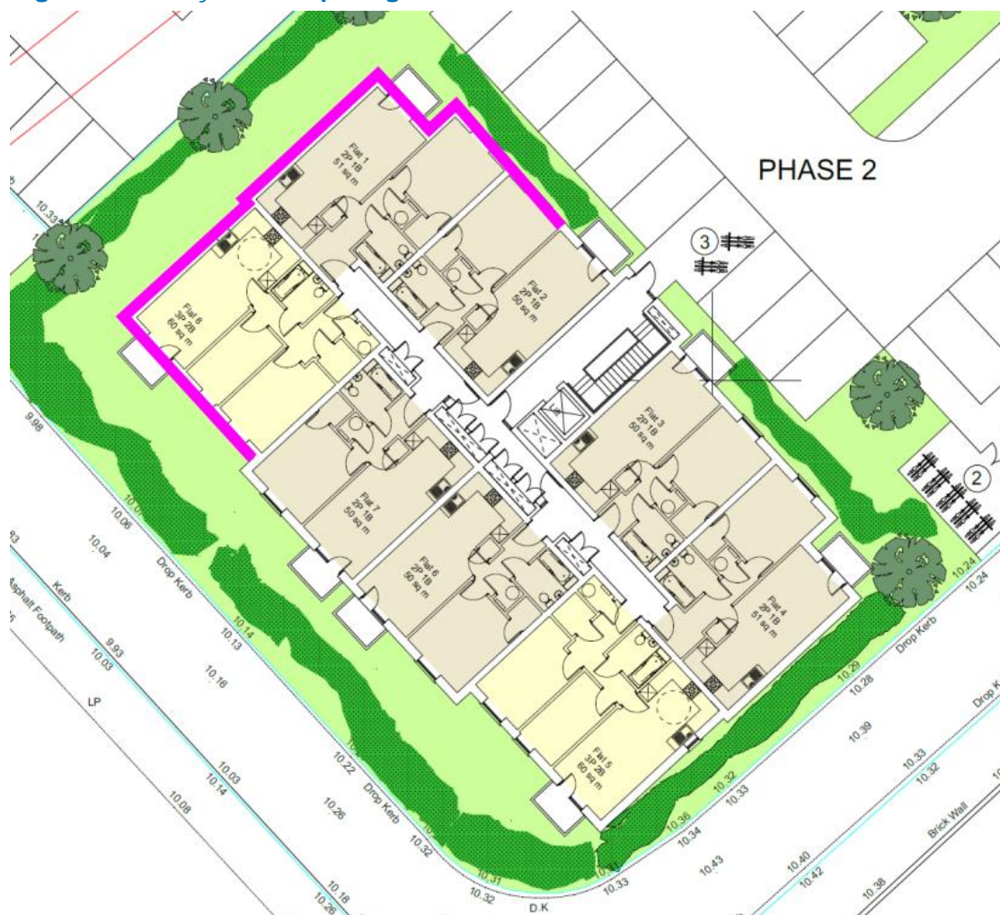
Figure 5.1 – Façades Requiring Additional Sound Insulation Measures
