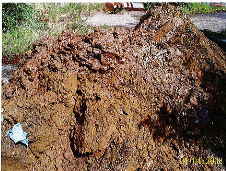
Photograph 12: Photograph showing arisings from TP4, materials with hydrocarbon sheen visible on top of spoil heap.
