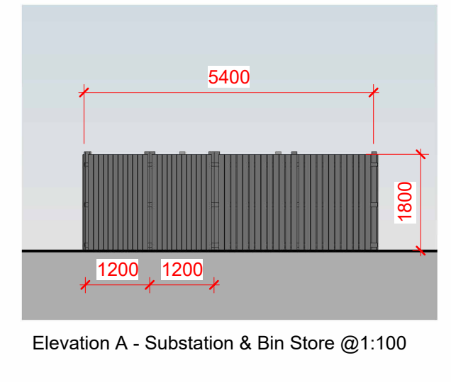
Elevation A - Substation & Bin Store @ 1:100
