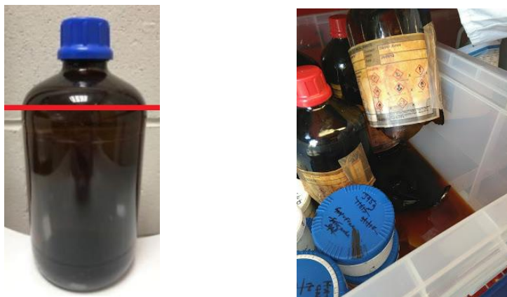
Figure 2 – Maximum fill height of a Winchester and the consequences of overfilling and incorrect use
