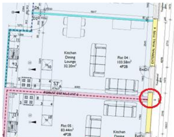
Figure 3.3 – Intersection of Party Wall & External Wall for Comment
