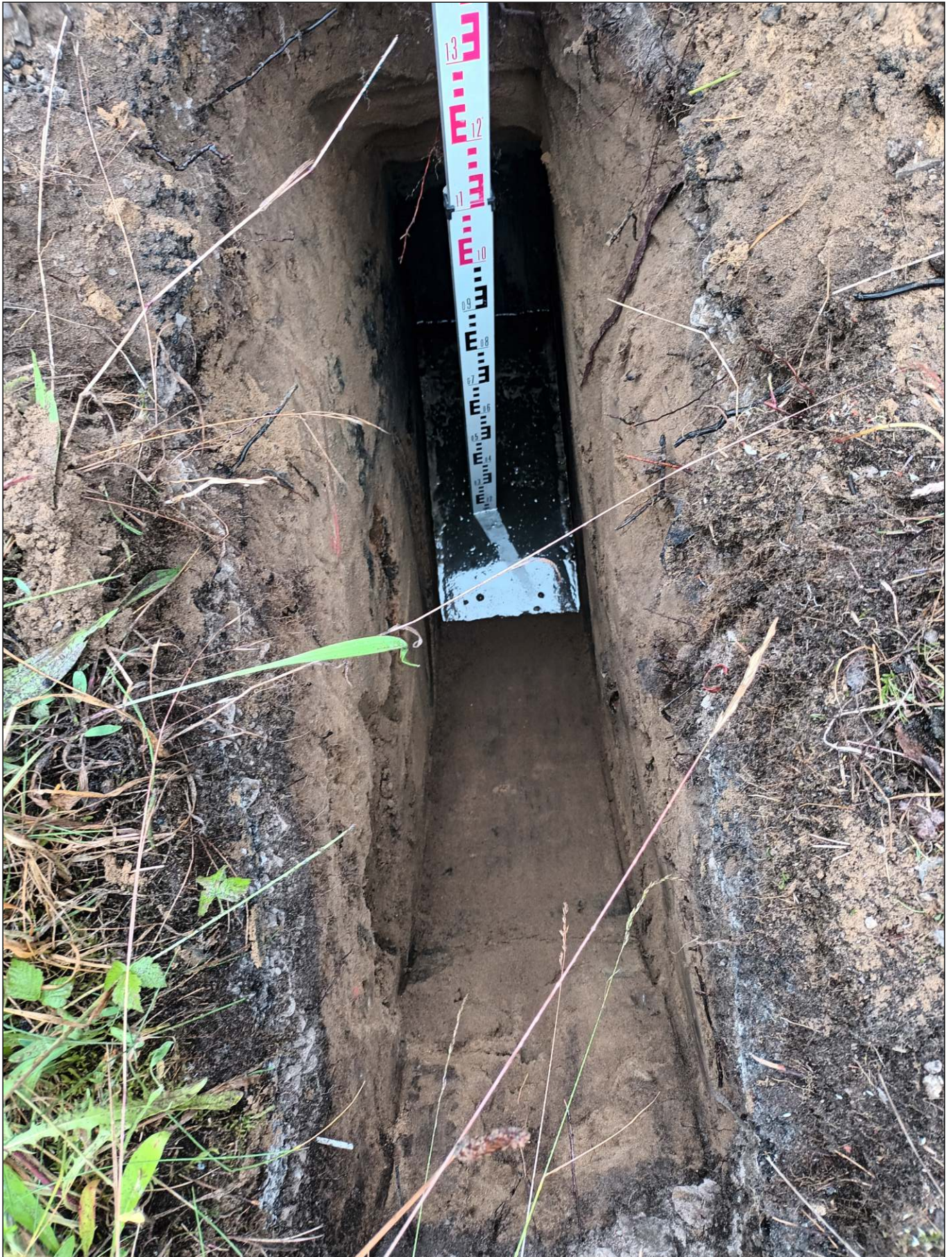
FIGURE 2 WATER TABLE AT 1.5m IN SA2.
