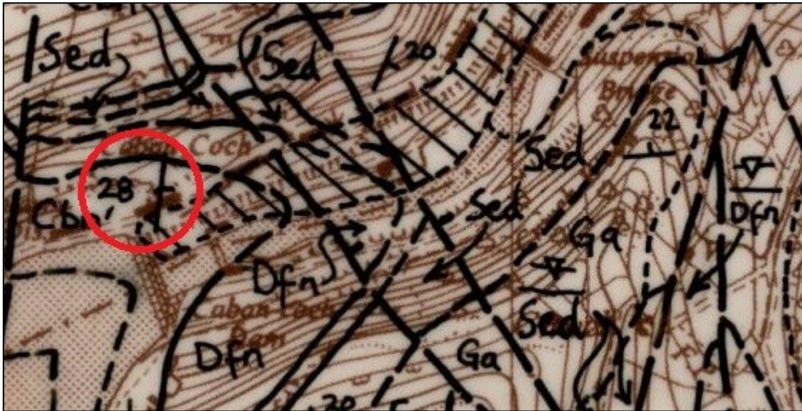
Figure 3: Extract from 1:10,000 scale geology map [5]. Narest recorded dip measurement circled in red.
