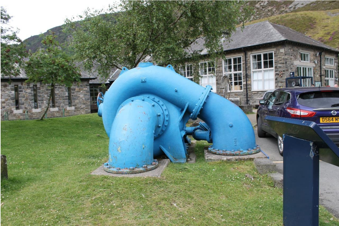
Image EDP A1.19: View illustrating the appearance of the hydro-electric turbine displayed outside the entrance to the Visitor Centre building
