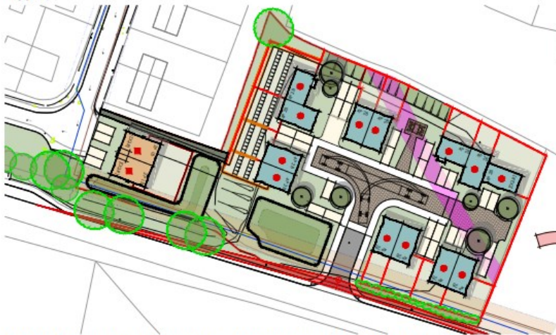
OPTION 4 - Consisting 17No dwellings with main access from A4059 with 4No dwellings at the lower level and accessed from Ger-Y-Bont. Existing Adit defines dwelling positions and steep access road up to main level of site. Hammer head adoptable road within central area of site offering access to all properties and a public realm. Sudds design to both upper an lower areas.
