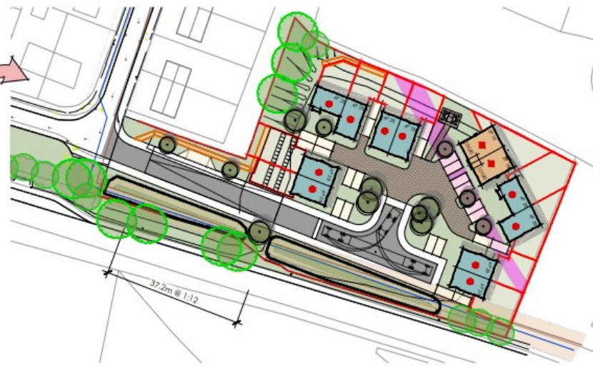
OPTION 2 - Consisting 14No dwellings with main access from the lower level of Ger-Y-Bont. Existing Adit defines dwelling positions and steep access road up to main level of site. Hammer head adoptable no within central area of site offering and properties access from shared surface courts.
