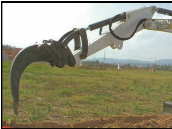
Plate 11: Excavator arm fitted with a Single Tine Ripper Attachment
