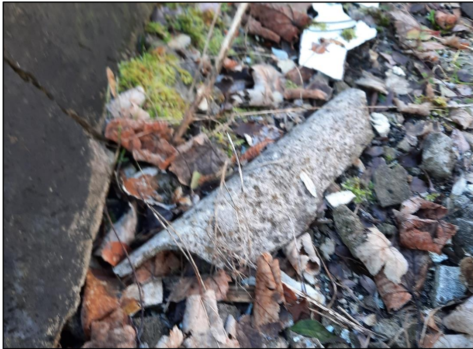
Plate 7: Asbestos Cement Sheet within Stockpile of Demolition Rubble (northern margins)
